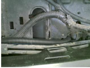
Route the fuse box cable to the fuse box and attach with the bolt supplied.
