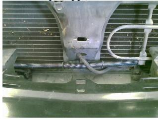
Route the fuse box cable through the hole below the driver side headlight.
