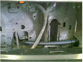
Route the fuse box cable along with the factory loom going across to the drivers side, attach with tie raps supplied.
