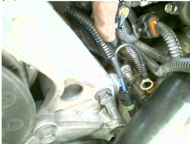
6. Plug the harness into the water pump plug. (“F”)
