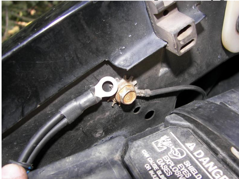
Ground wire going to fender bolt.
