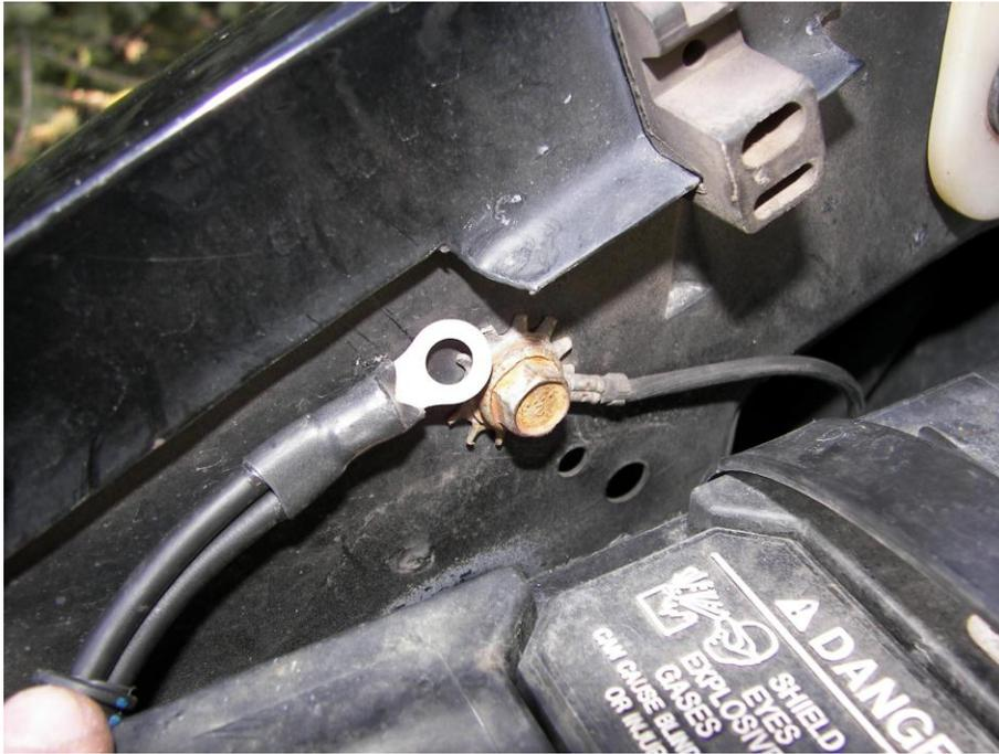
17. Route the fan ground wires over to the ground bolt on the fender #10.
