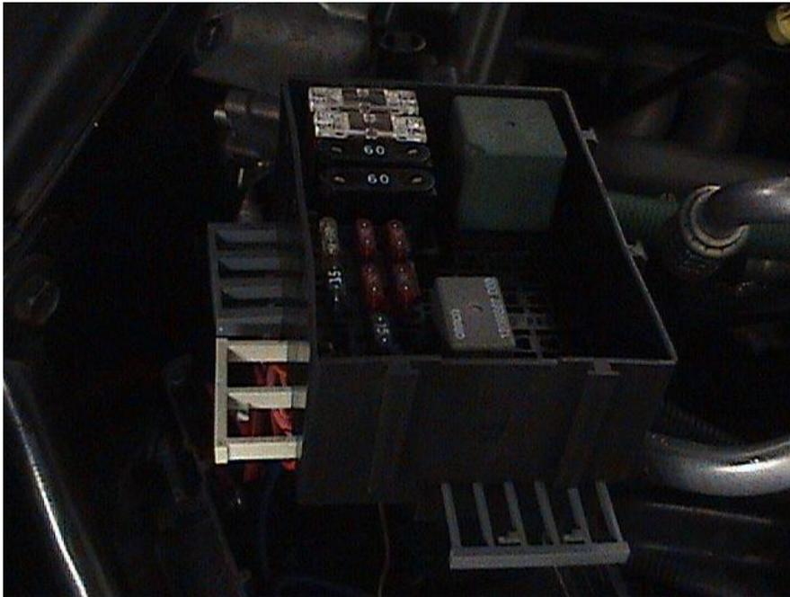
**Remove the three retaining clips from the fuse box.**
